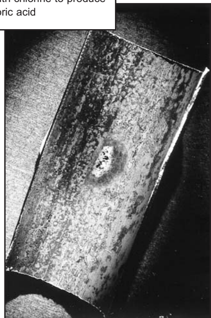
Figure 9: Crevice corrosion under bacteria colony on the inside of a stainless steel tube (magnification 5X)
